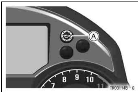
A. Oil Pressure Warning Indicator Light
